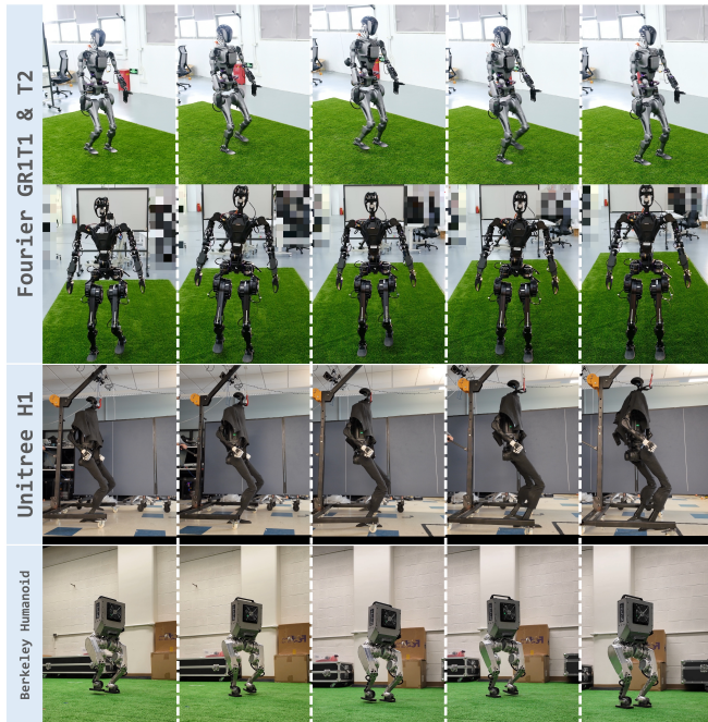
Fig. 7: Real-world deployment. LCP is able to train effective locomotion policies on a wide range of robots, which can be directly transferred to the real world.
